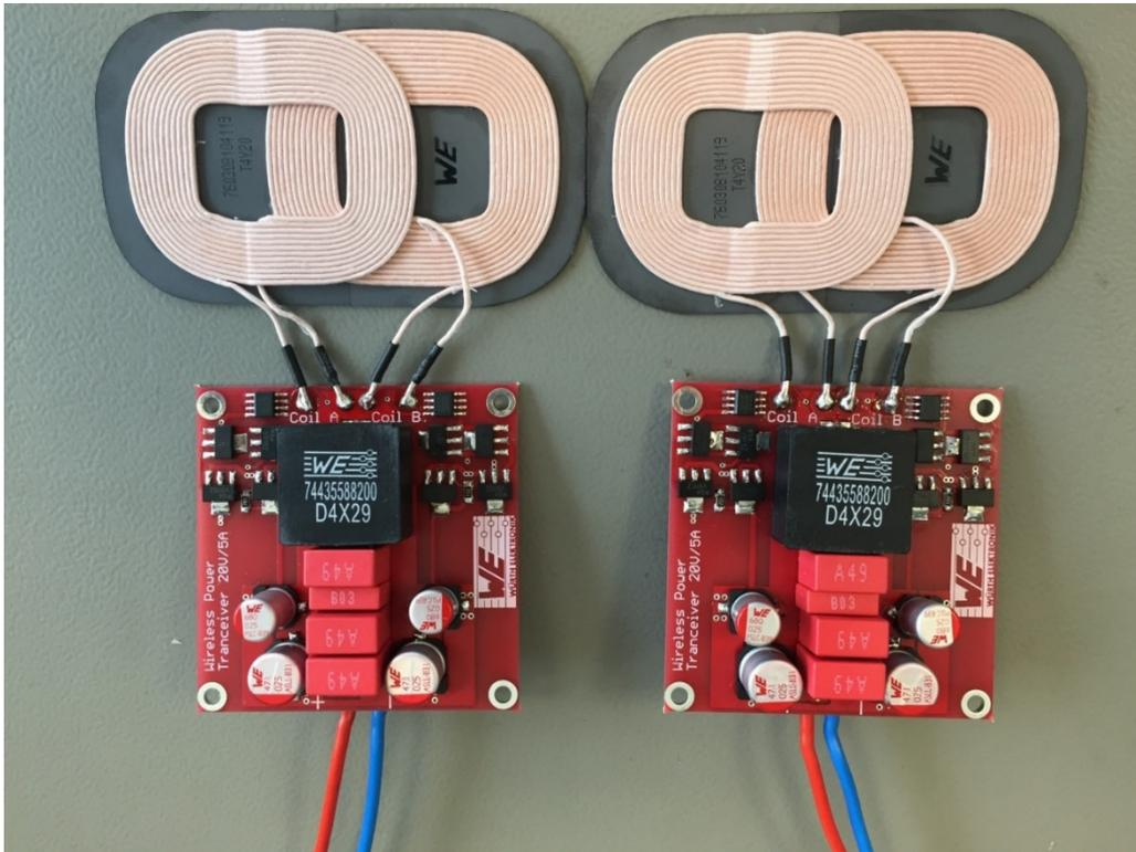
Figure 22: Construction for application example transmitter/receiver 3.9 for coil array ([760 308 104 119](https://www.wuerth-elektronik.com/760308104119)).
