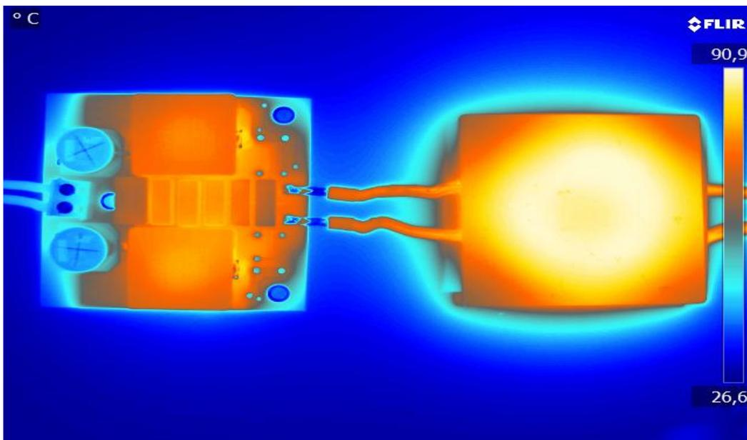
Figure 8: Temperature rise (upper side = filter + capacitors) of the circuit/coils for  $P_{out} = 100 \text{ W}$  ( $V_{in} = 20 \text{ V}$ )
