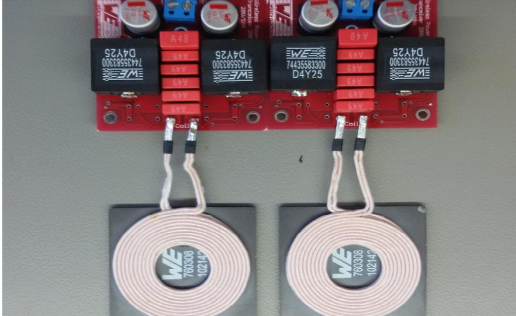
Figure 7: Measured circuit ( $V_{in} = 20 \text{ VDC}$ ;  $P_{out} = 100 \text{ W}$ ) for a 6.5 mm air gap
