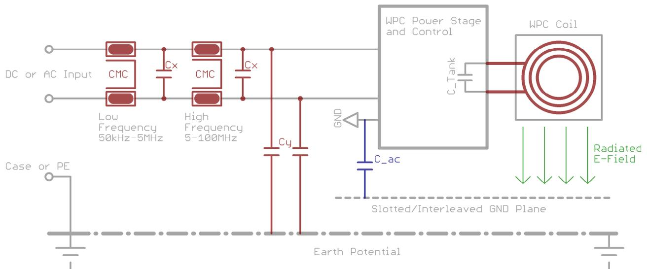
**Figure 11: Measures for containment of common mode and differential mode interference sources**
