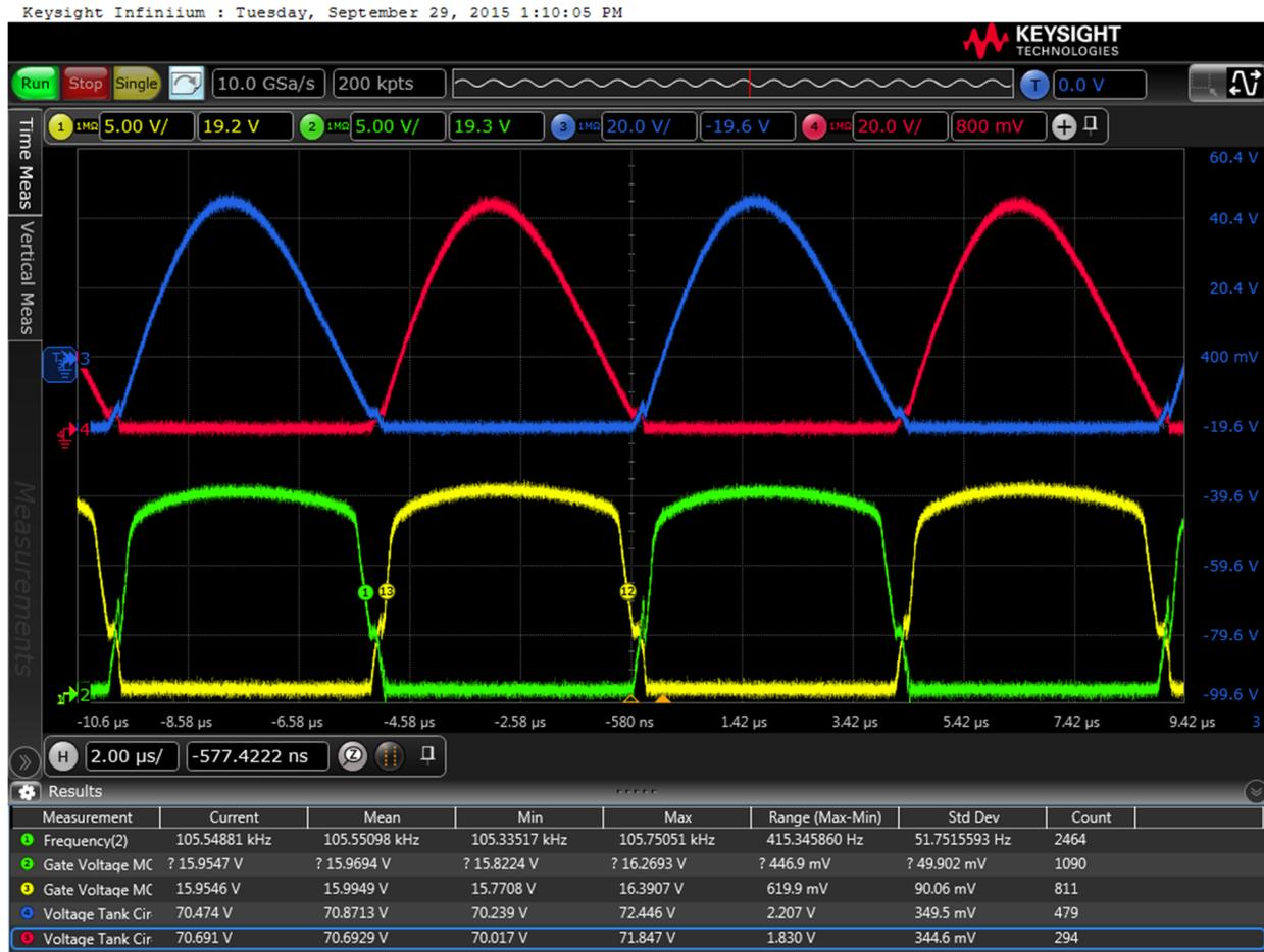
**Figure 3: The voltages at the transmitter coil are shown in blue and red. The gate voltages are yellow and green (These measured voltage curves are referenced to the circuit ground GND;  $V_{in} = 20\text{ V}$ ;  $P_{out} = 100\text{ W}$ ; optimized gate drive, see application examples)**
