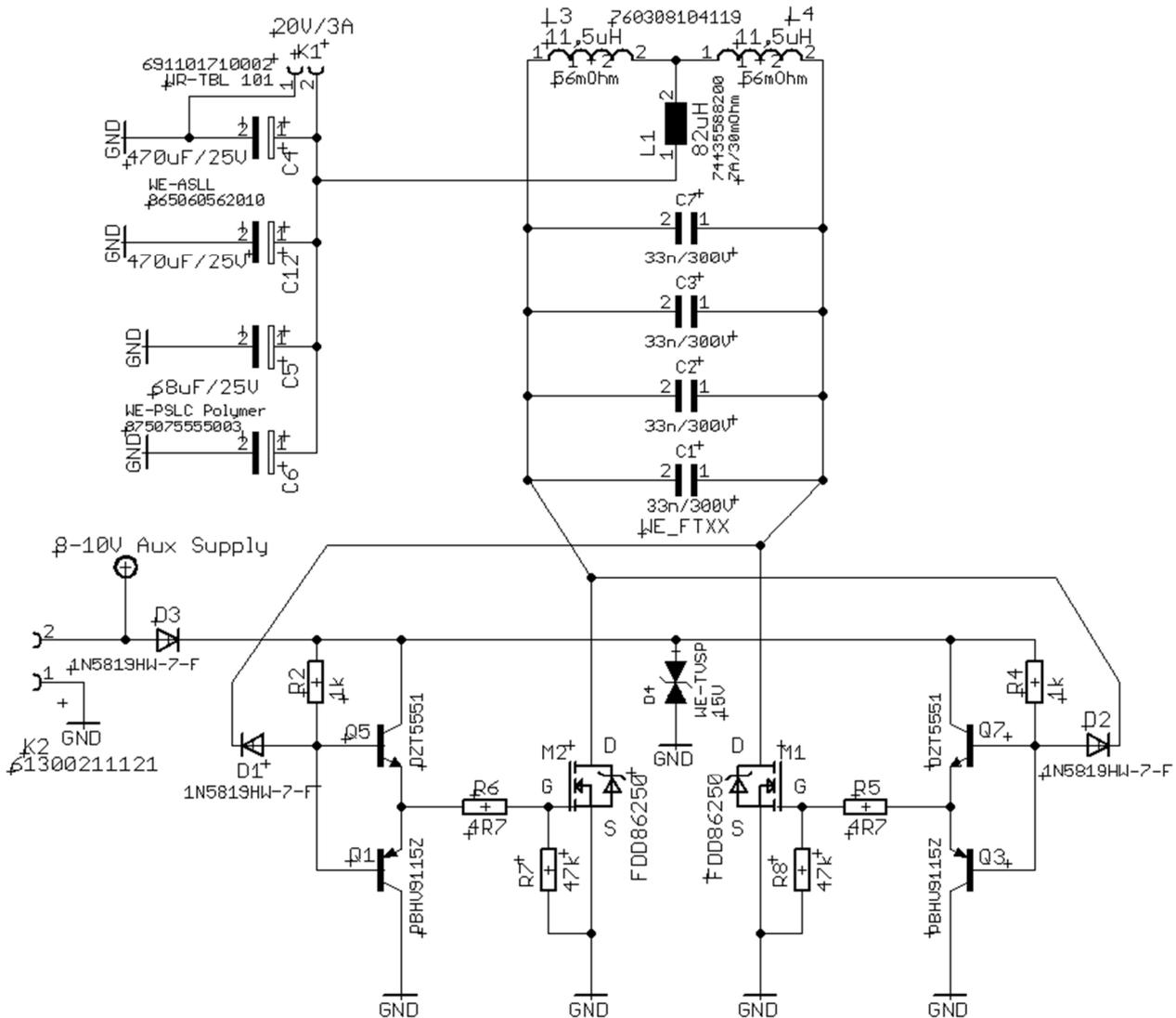
**Figure 21: Resonance converter for coils with center tap. The advantage of the circuit is that you only need one filter coil. Due to the center tapping, the frequency is twice as high and the voltage swing is reduced. This allows smaller filter coils to be used. In addition, an array with two overlapping coils can be easily controlled. The 8 - 10 V auxiliary voltage can be generated from the operating voltage using an LDO or WE Magic Power Module ([171 012 401](#)).**
