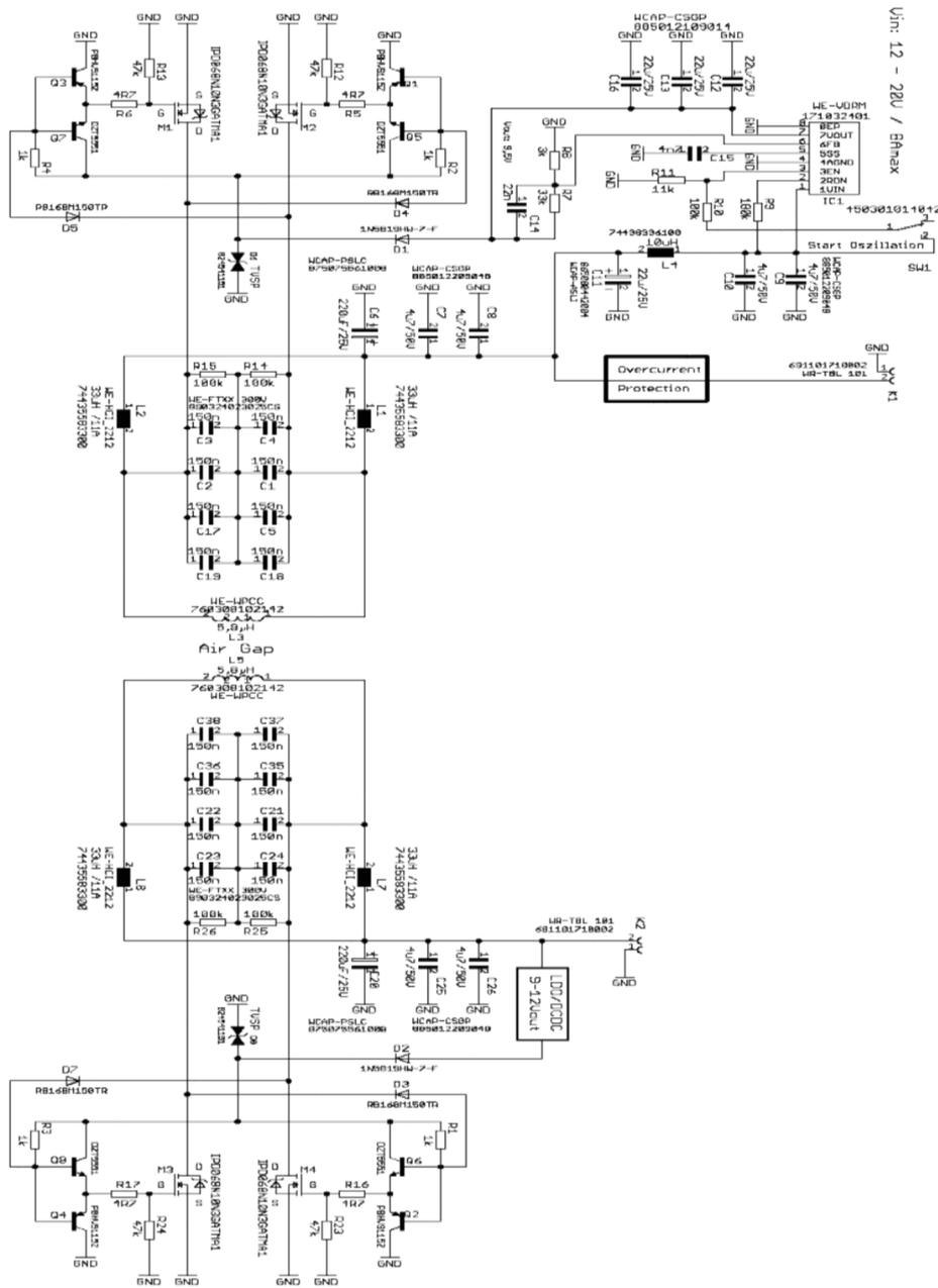
Figure 20: Transmitter and receiver for approx. 100W.
