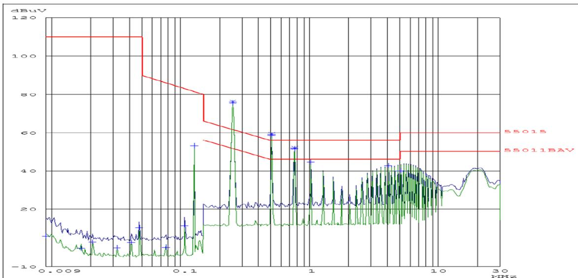
Figure 10: Example for a spectrum in interference voltage measurement (9 kHz - 30 MHz / Limit Class B)
