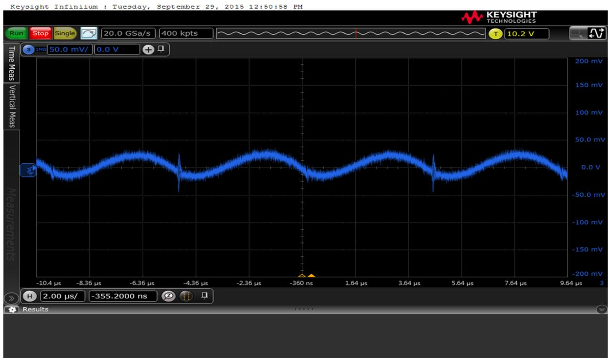
Figure 5: Reflected voltage ripple and noise to supply the input on the transmitter side ( $V_{in} = 20\text{ V}$  /  $P_{out} = 100\text{ W}$ ) → Polymer and ceramic capacitors with a low ESR can be used to reduce the voltage ripple.
